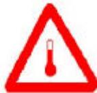
5.3.2.2.2 In addition to the elevated temperature mark, the maximum temperature of the substance expected to be reached during transport shall be durably marked on both sides of the portable tank or insulation jacket, immediately adjacent to the elevated temperature mark, in characters at least 150 mm high.
